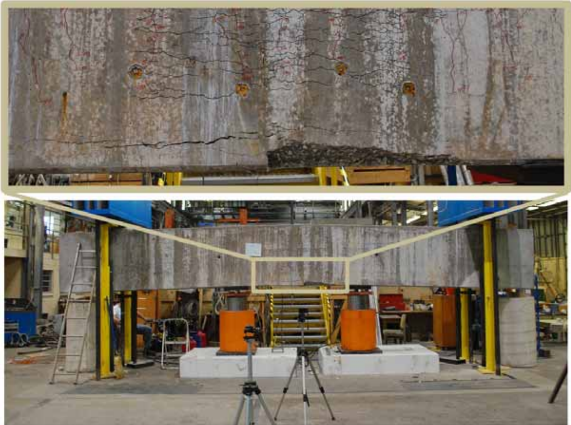
Figure 7.10: Crushing failure, first reactive specimen.
