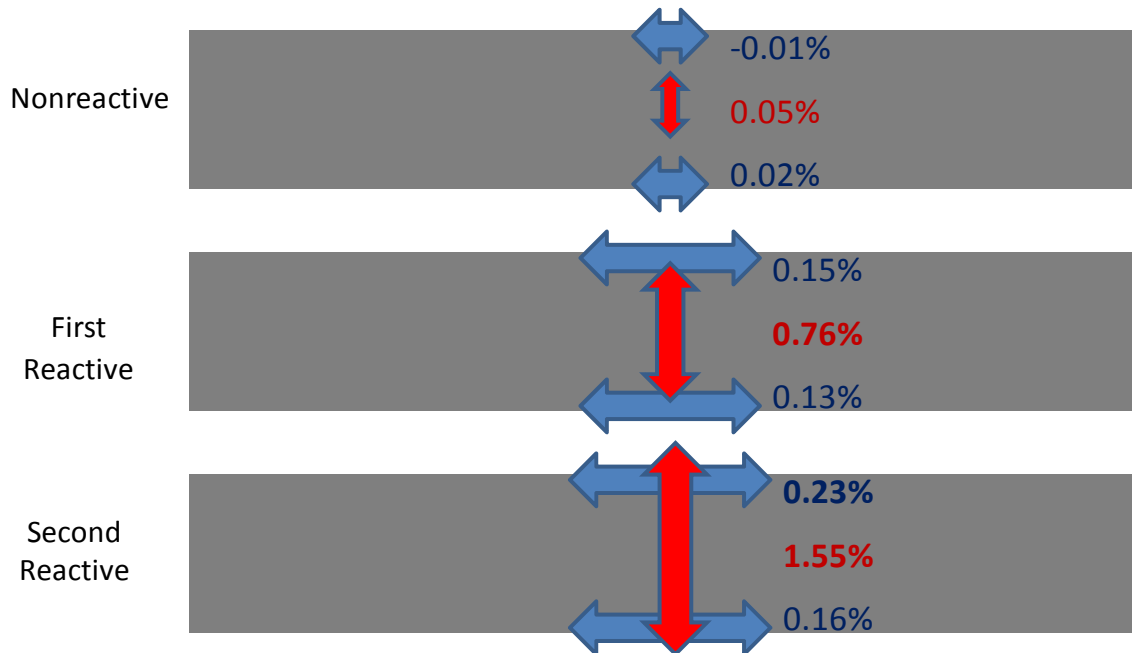
Figure 7.1: Expansions of specimens after removal of conditioning load.
