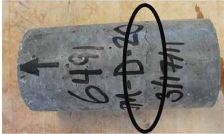
Figure 4.5: DEF cylinder with open crack at surface.
