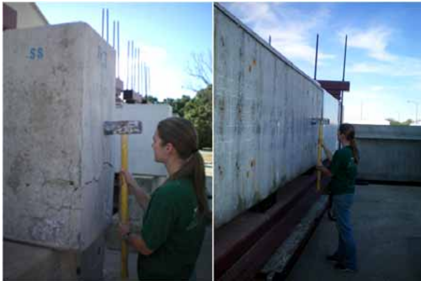
Figure 5.19: Impacts for dynamic testing of beam specimen.
