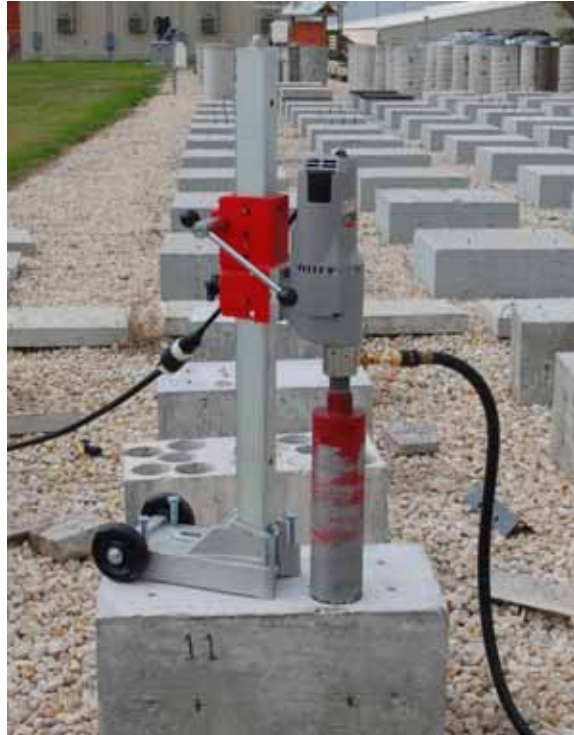
Figure 3.16: Coring rig mounted on exposure block.
