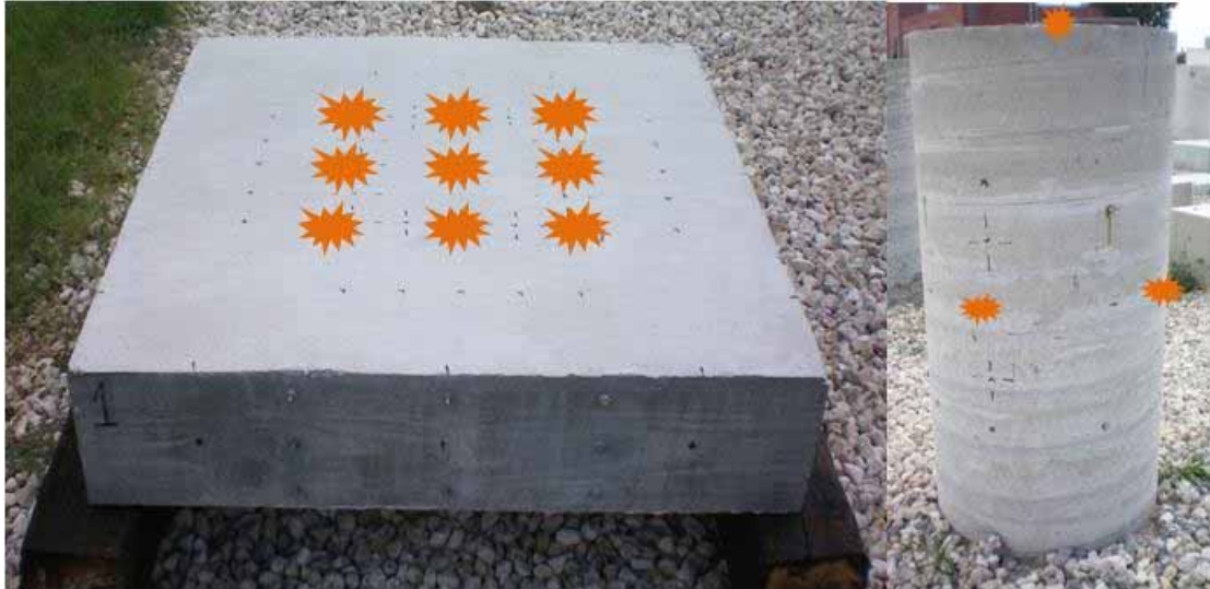
Figure 3.13: Impact-echo locations for bridge deck and column.
