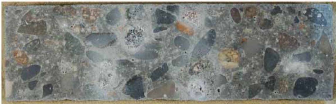
Figure 2.18: Gel pat test specimen at 56 days, from Fournier 2009.
