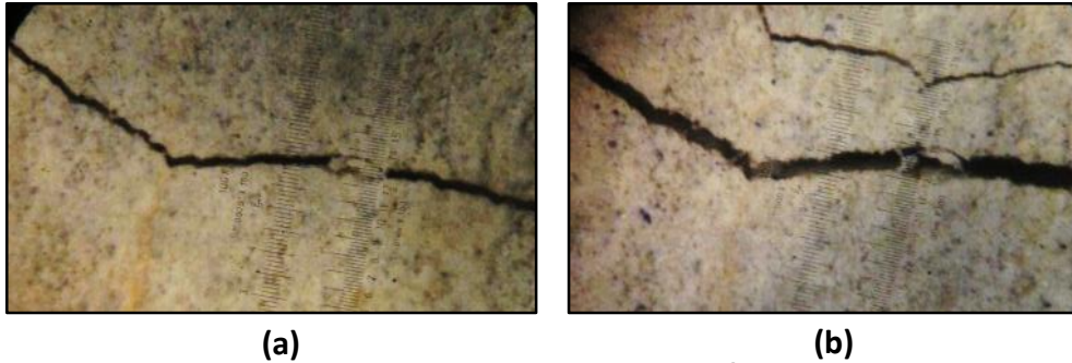
Figure 3.21 – Crack width: (a) at first cracking (width \approx 1 \times 10^{-3} in.), (b) at extensive cracking (width \geq 3 \times 10^{-3} in.)
