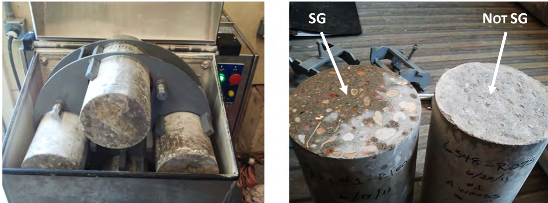
Figure F-62: Surface-grinding (SG) uneven faces of test specimens
