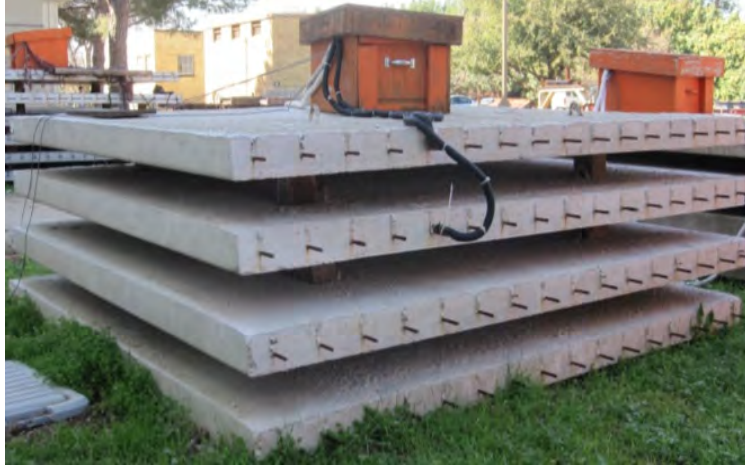
Figure 2-15: Long-term monitoring of prestress loss in PCPs
