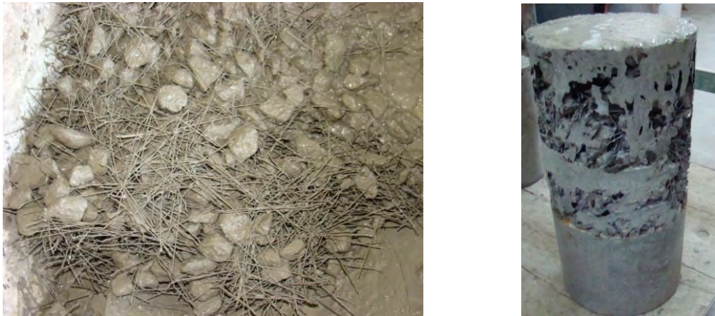
Figure F-8: Examples of mixing difficulties in Phase 1 with high fiber-volume fractions
