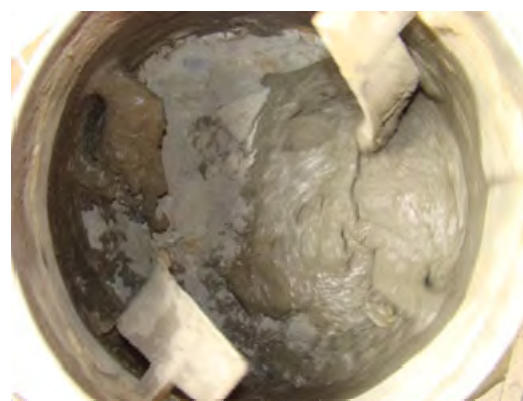
Figure F-2: Typical procedure for mixing concrete: (a) batching of materials; (b) gradual addition of water to prepare workable paste
