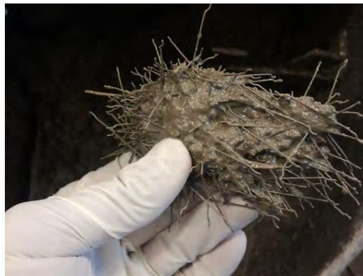
Figure F-56: Example of “clumping” and “balling” of fibers observed during mixing
