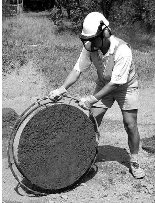
Figure E-11: Rolling steel form after molded specimen has gained sufficient strength (ASTM C1550 2010)
