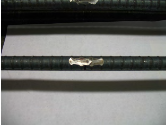
(a) Grind surface of reinforcing bar
