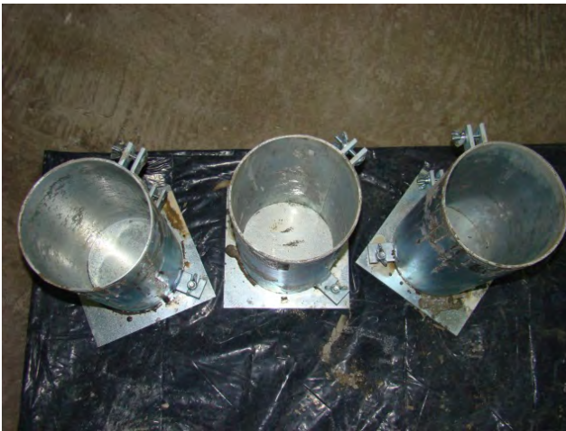
Figure F-9: Steel molds used to prepare specimens in Phase 3 at UT Arlington
