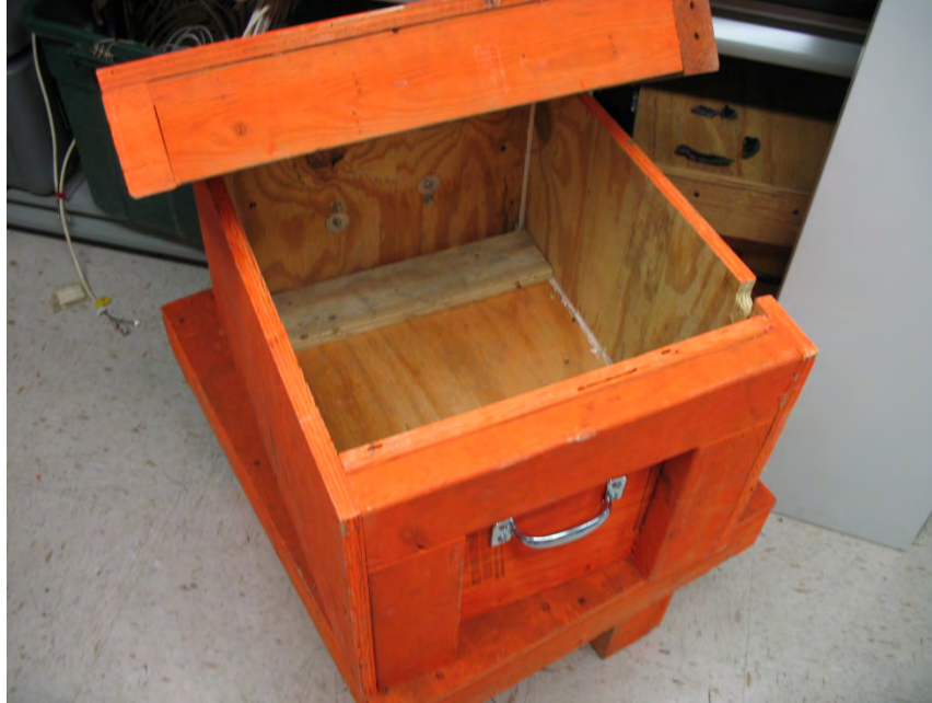
Figure 6-8: Wooden box for data logger
