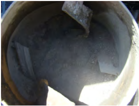
Figure F-2: Typical procedure for mixing concrete: (a) batching of materials; (b) gradual addition of water to prepare workable paste
