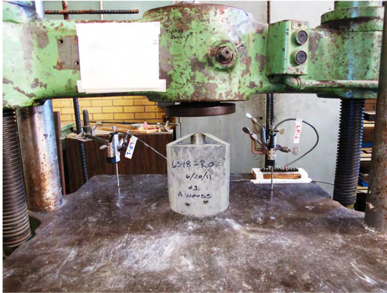
Figure F-65: DPT setup on 60-kip Baldwin UTM (hydraulic)
