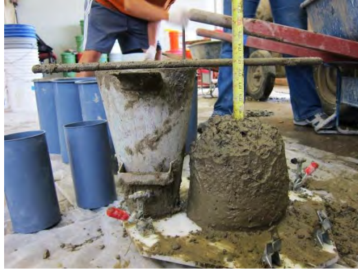
Figure F-57: SFRC mixing sequence, Step 6
