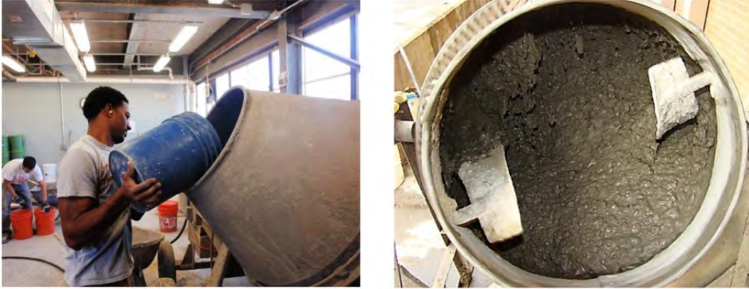
Figure F-54: SFRC mixing sequence, Step 4
