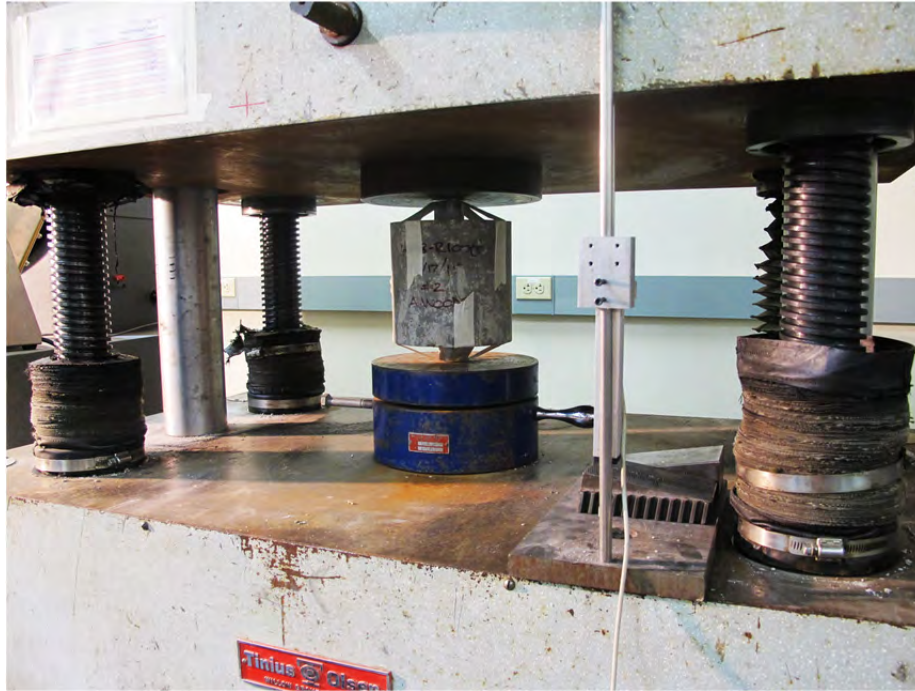
Figure F-67: DPT setup on 120-kip Olsen UTM (screw-type)
