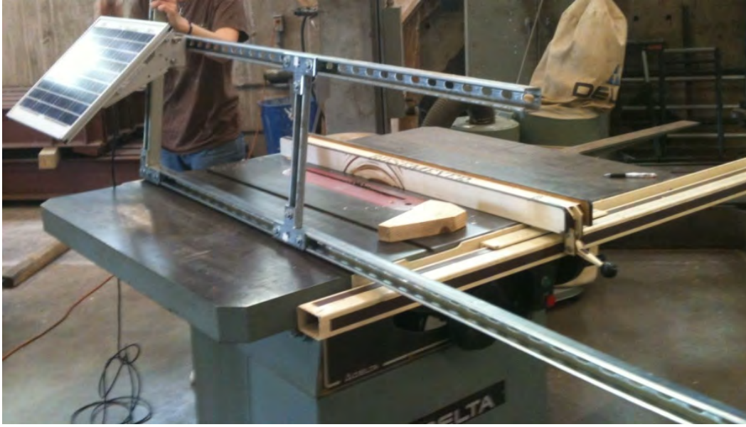
Figure 3-16: Bracket for solar panel, Wharton-Weems Overpass
