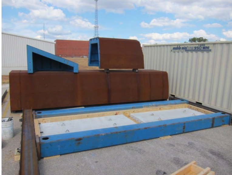
Figure 4-9: Complete assembly of first bay, restrained-shrinkage test
