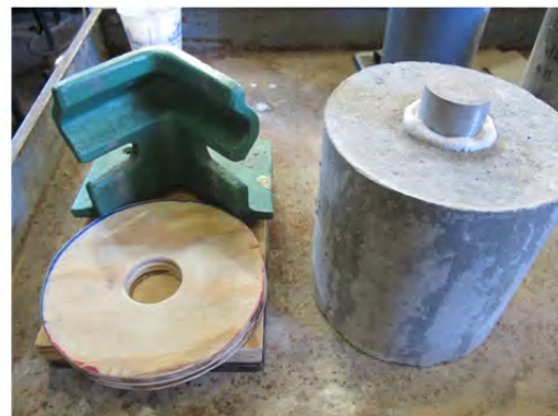
Figure F-63: Process of applying hydro-stone to rough faces of test specimen
