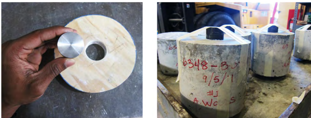
Figure 5-12: Steel punch centering guide and masking tape used to secure against eccentric loading effects
