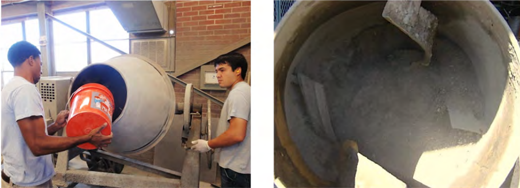
Figure F-52: SFRC mixing sequence, Step 2
