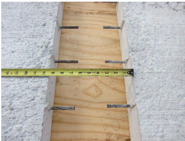
Figure 4-10: Space between PCPs, restrained-shrinkage test
