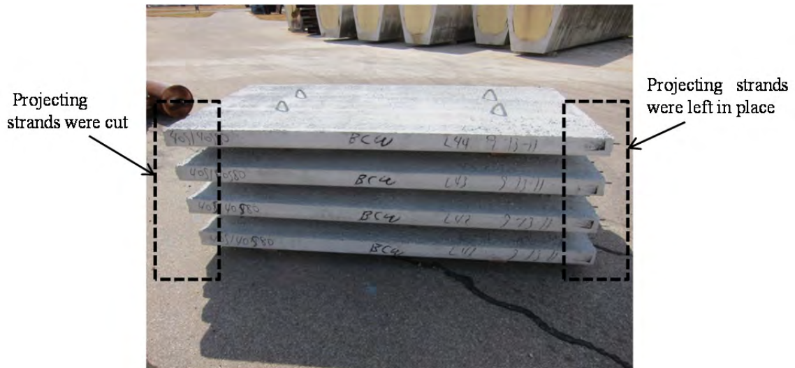
Figure 4-7: Half-size precast, prestressed concrete panels (strands cut on one side)
