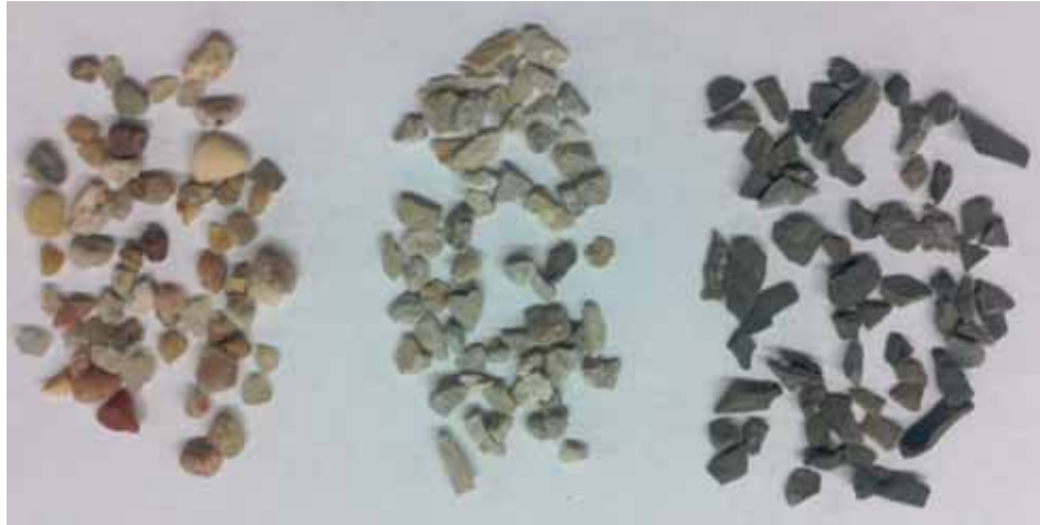
Figure 6.1: Aggregates Retained on the No. 8 sieve (from left to right: Colorado River Sand, Hanson Perch Hill, and Lattimore Stringtown)
