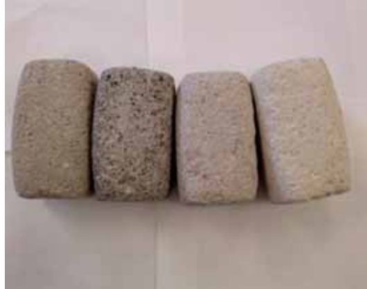
Figure 5.18: Larger Mortar Specimen For Testing Polish Resistance
