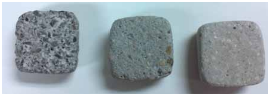
Figure 5.15: Mortar Specimen Tested for Texture (from left to right: Lattimore Stringtown, Colorado River Sand, and Texas Crushed Stone)
