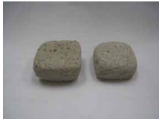
Figure 5.10: Mortar Brownies Made with Siliceous Sand at a Water-to-cement Ratio of 0.45 and 0.6
