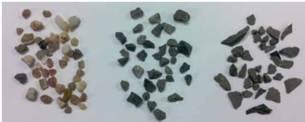
Figure 6.3: Aggregates Retained on the No. 8 sieve (from left to right: Colorado River Sand, Lattimore Stringtown (Metso 65 m/s), and Lattimore Stringtown)
