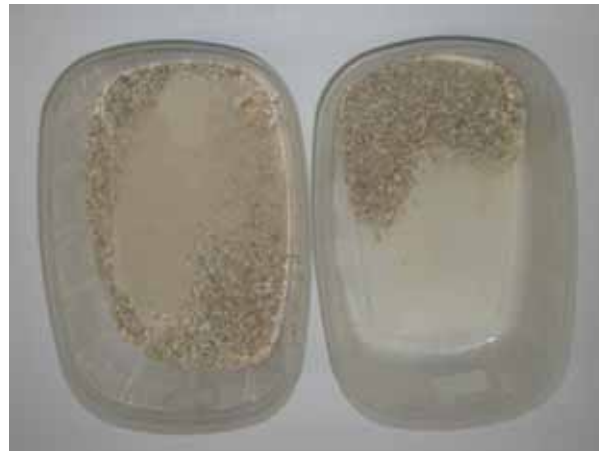
Figure 5.3: Hanson Servtex Before and After Micro-Deval (120 Minutes Run time)
