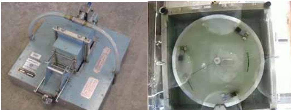
Figure 8.2: Dynamic Friction Tester
