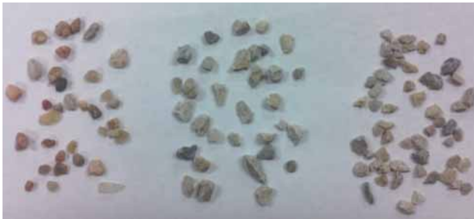
Figure 6.2: Aggregates Retained on the No. 8 sieve (from left to right: Colorado River Sand, Hanson Perch Hill (Metso 60 m/s), and Hanson Perch Hill)
