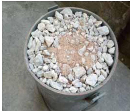
Figure 7.11: Example of a Combined DRUW Test
