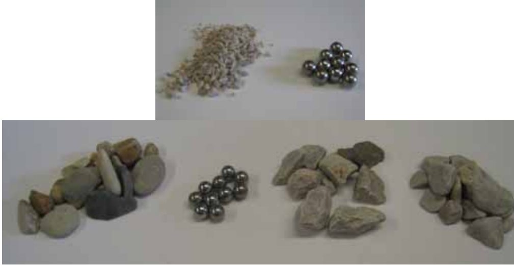
Figure 5.4: Fine and Coarse Aggregate Sizes Compared to 10mm Ball Bearings
