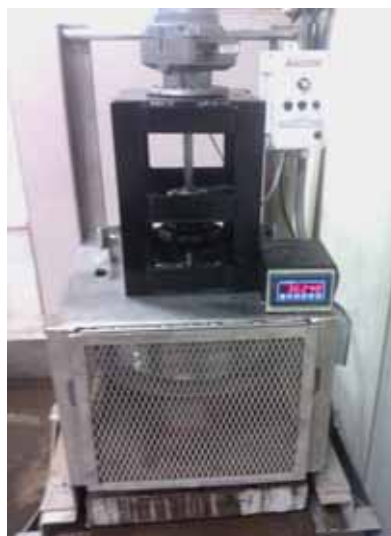
Figure 10.2: Modified Three-Wheel Polishing Device
