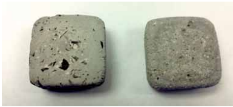
Figure 5.16: Abraded Lattimore Stringtown and Colorado River Sand Mortar Specimens
