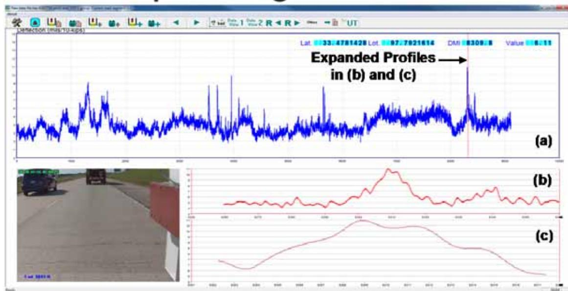
Figure 3.5: Area High Deflection Area Not Associated with a Patch
