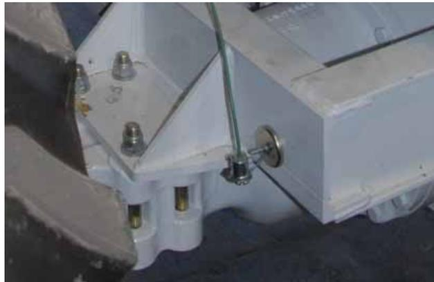
*Figure A.20: Infrared Sensor for Getting the Surface Temperature*
