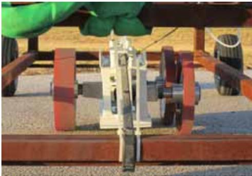
(a) SA: 9.5-in. Diameter Wheels: Two, 1-in. and One, 2-in. Wide Treads
